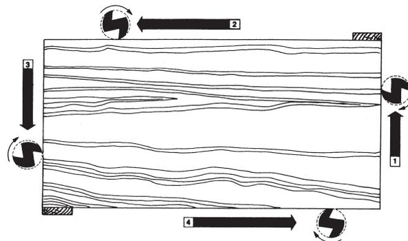
**Figure 37-14: Routing Work Around Outside Edges**
