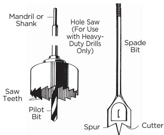
**Figure 37-4: Drill Attachments that Require Control by Operator**
