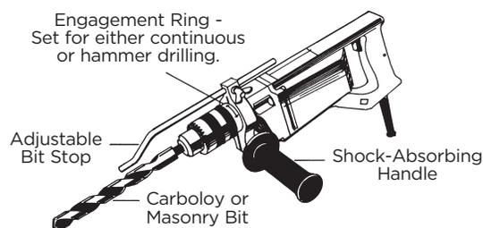
**Figure 37-5: Impact or Hammer Drill**
