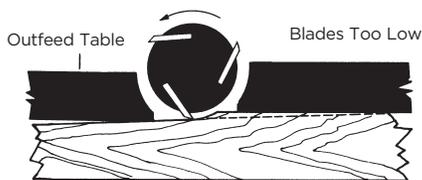
When cutter blades are installed lower than the level of the outfeed table, the plane hobbles over the material and the cut is uneven.
