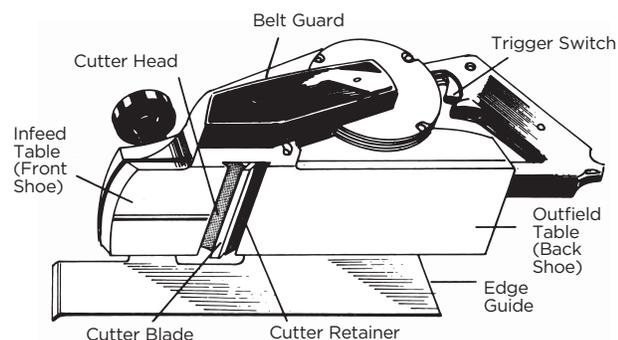
**Figure 37-9: Standard Power Plane**
