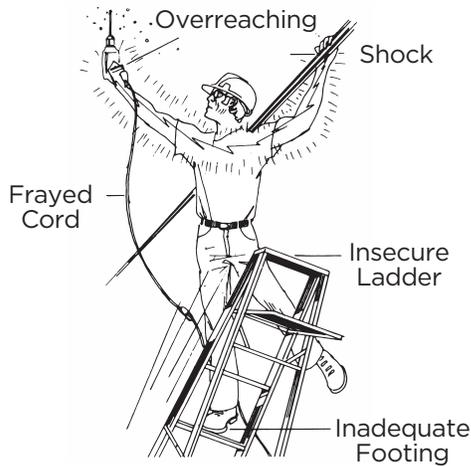
**Figure 37-7: Drilling and Ladder Hazards**
