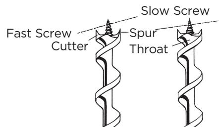
**Figure 37-8: Self-Feeding Auger Bits**
