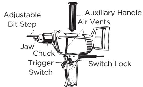
Figure 37-2: Heavy-Duty Drill
