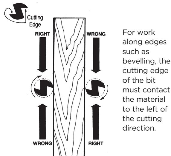
For work along edges such as beveling, the cutting edge of the bit must contact the material to the left of the cutting direction.
