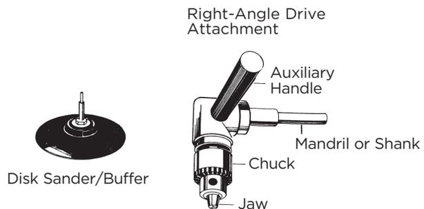
Figure 37-3: Drill Attachments
