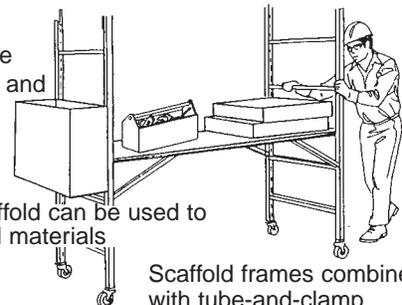
A small rolling scaffold can be used to transport tools and materials.
