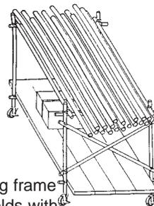
Rolling frame scaffolds with tube-and-clamp components can be used to move pipe and other material.
