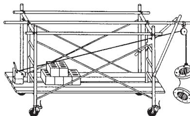
Scaffold frames combined with tube-and-clamp components, casters, and a small boat winch have many uses in moving and lifting.
