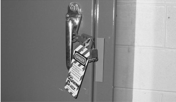
Lockout and tagging ensures that hazardous energy sources are under the control of each worker. Serious or fatal accidents can occur when people assume that machinery is turned off or made harmless—but it isn't.
