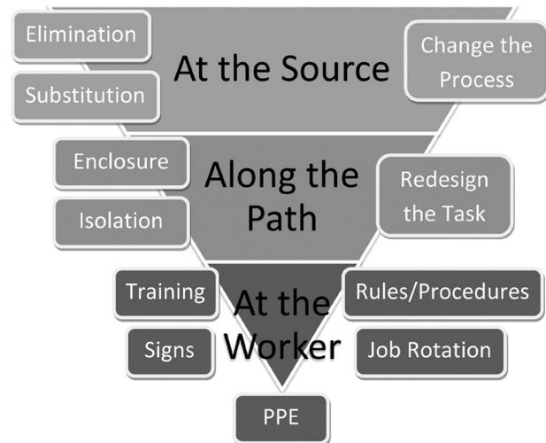
Figure 10-1: Hierarchy of Controls
