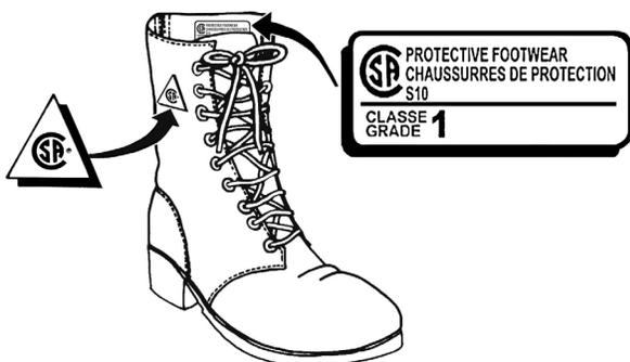
Figure 13-1: Grade 1 Safety Boot with CSA Label
