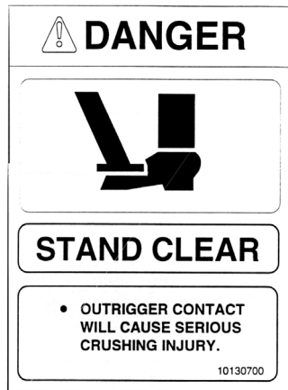
Figure 22-11: Typical Warning Sign
