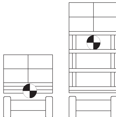
Figure 22-8 Centre of Gravity on Scissor-Type Lifts
