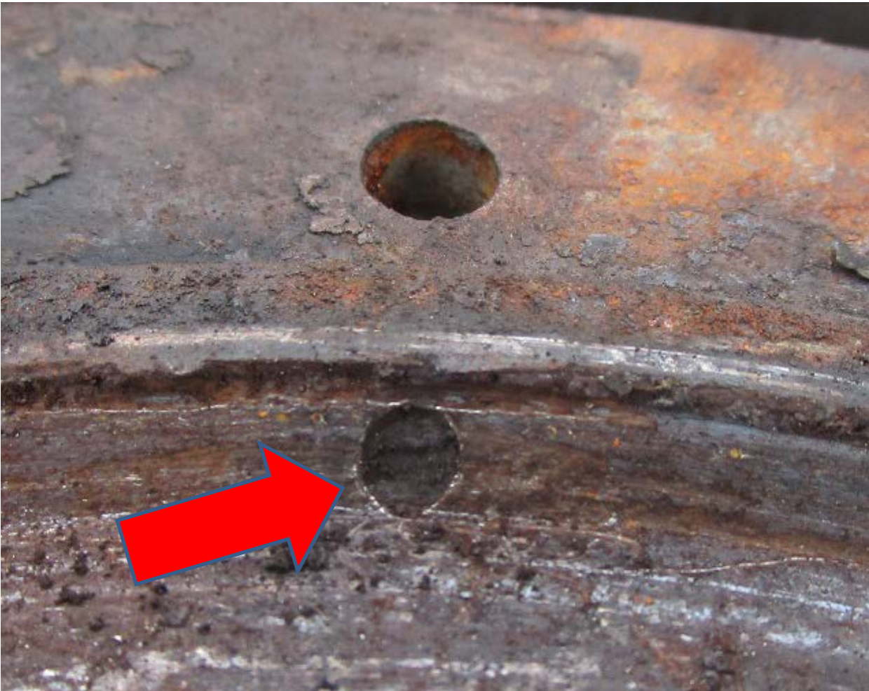
Lubricating oil supply system to bearing
