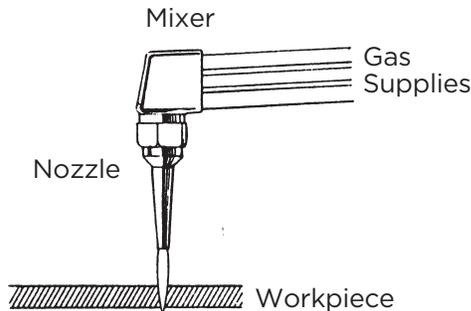
**Figure 41-5: Oxyacetylene Welding**
