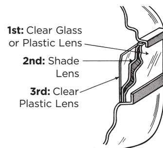
**Figure 41-16: Typical Lens Assembly for Arc Welding**
