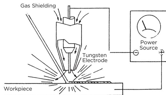
**Figure 41-4: Gas Tungsten Arc Welding**
