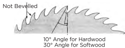
Figure 38-6: Ripsaw Blade
