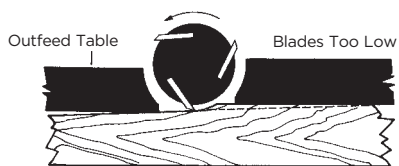
When cutter blades are installed lower than the level of the outfeed table, the plane hobbles over the material and the cut is uneven.
