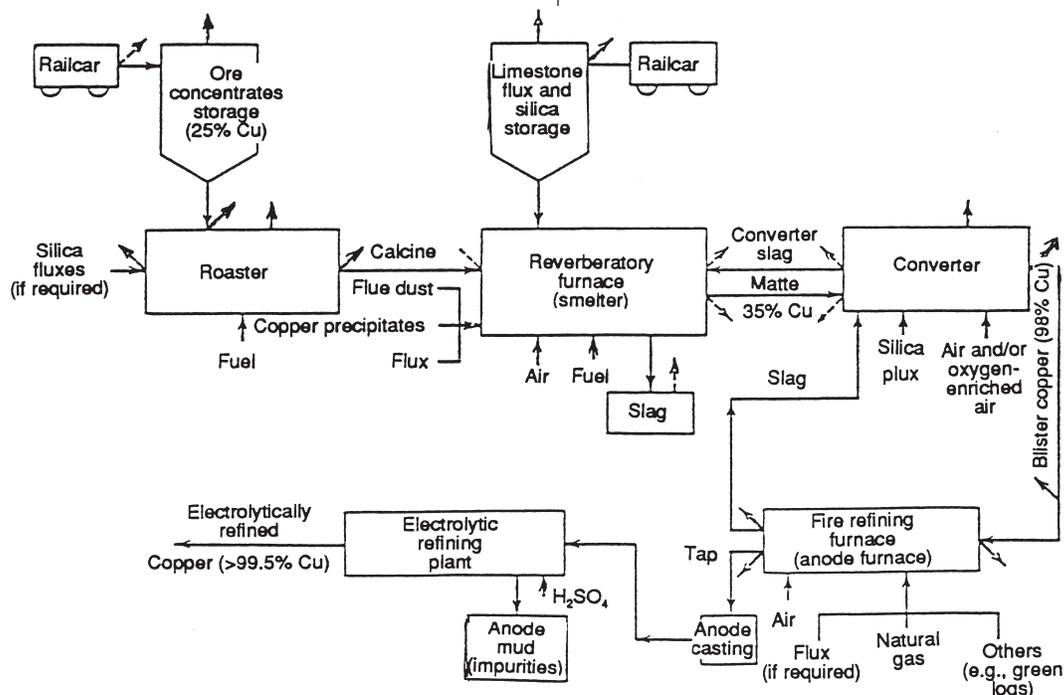
Figure 24.1 – Flow diagram for typical copper smelting operation
