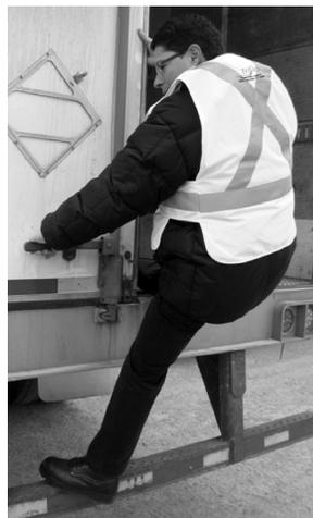
**Figure 30-5: Maintain Three-Point Contact**
