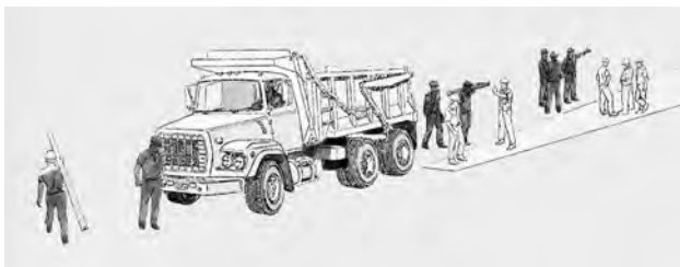
Figure 28-6: Workers in Blind Spots
