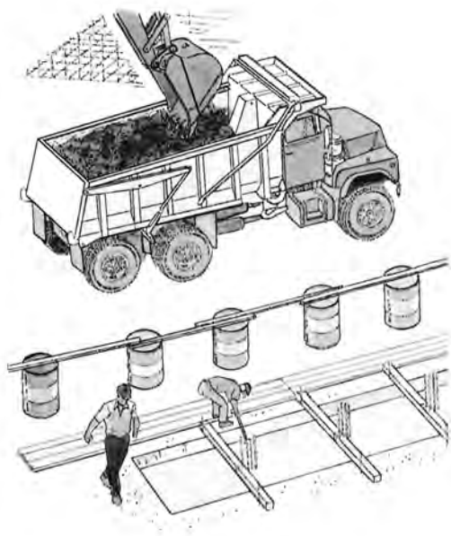
Figure 28-3: Use Barricades to Protect Workers
