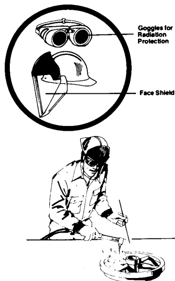
Figure 11-11: Protection from Heat, Glare, Sparks, and Splash (Brazing)
