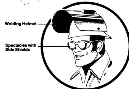
**Figure 11-16: Protection from Injurious Radiation (Electric Arc Welding)**
