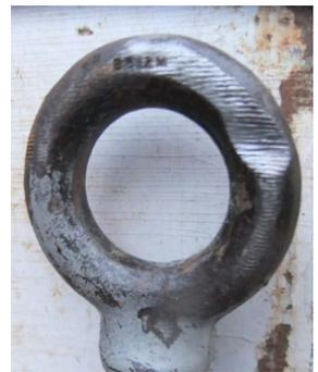
**Location of Eye Bolt and Close-up of Deterioration Caused by Wire Rope Abrasion**
